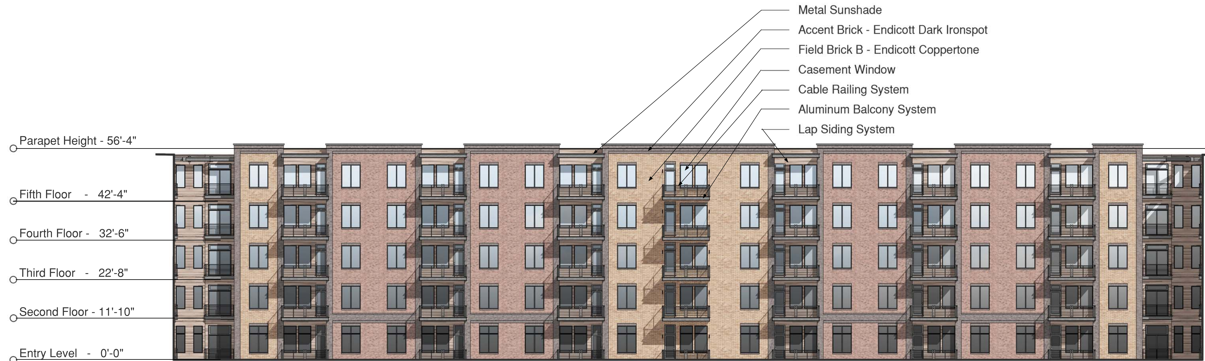
South Courtyard Elevation 1/16" = 1'-0"
