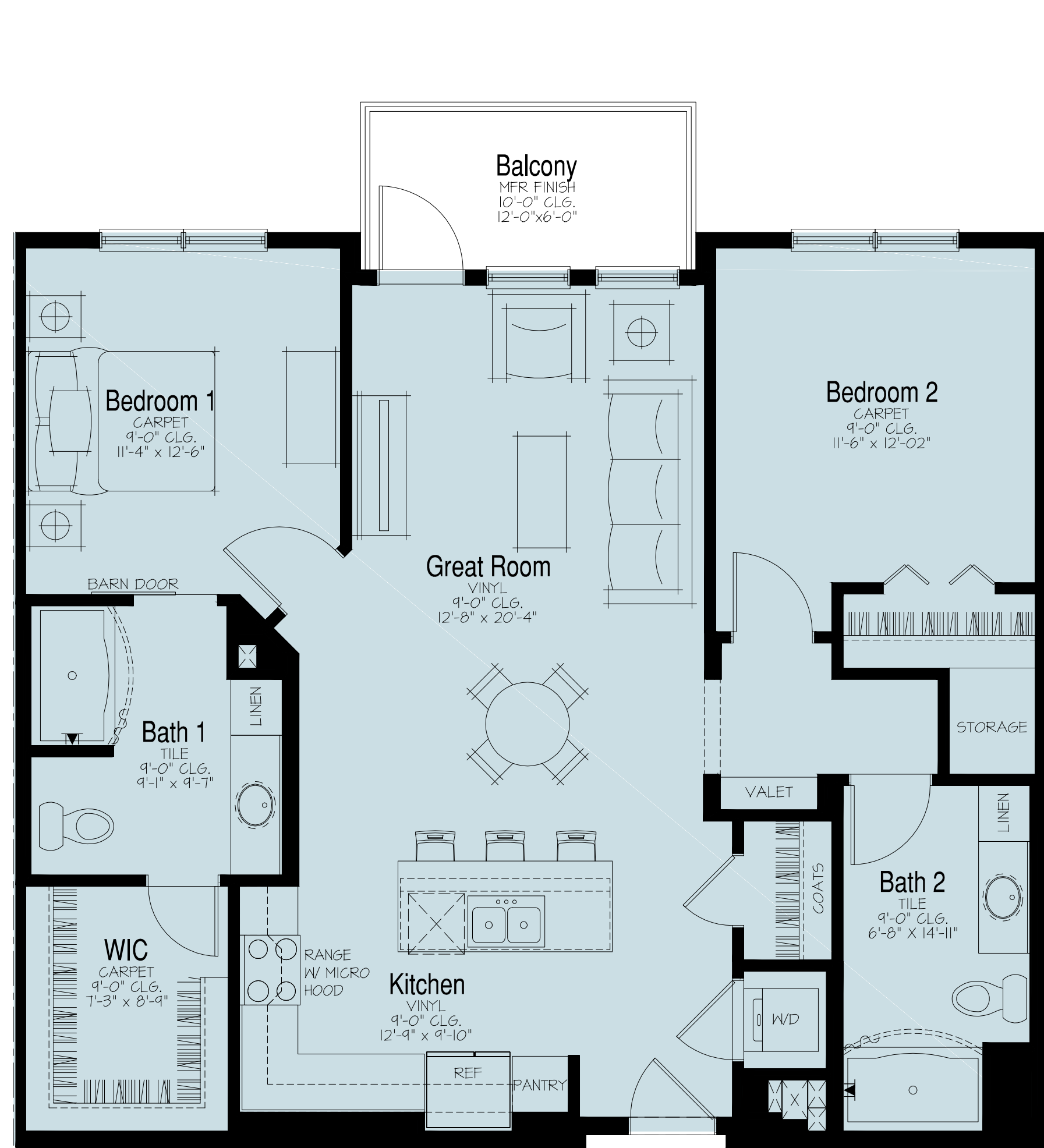
ANSI Type B: 2 Bedroom / 2 Bath NSF: 1111 / GSF: 1189 Unit - B1 Floor Plan
