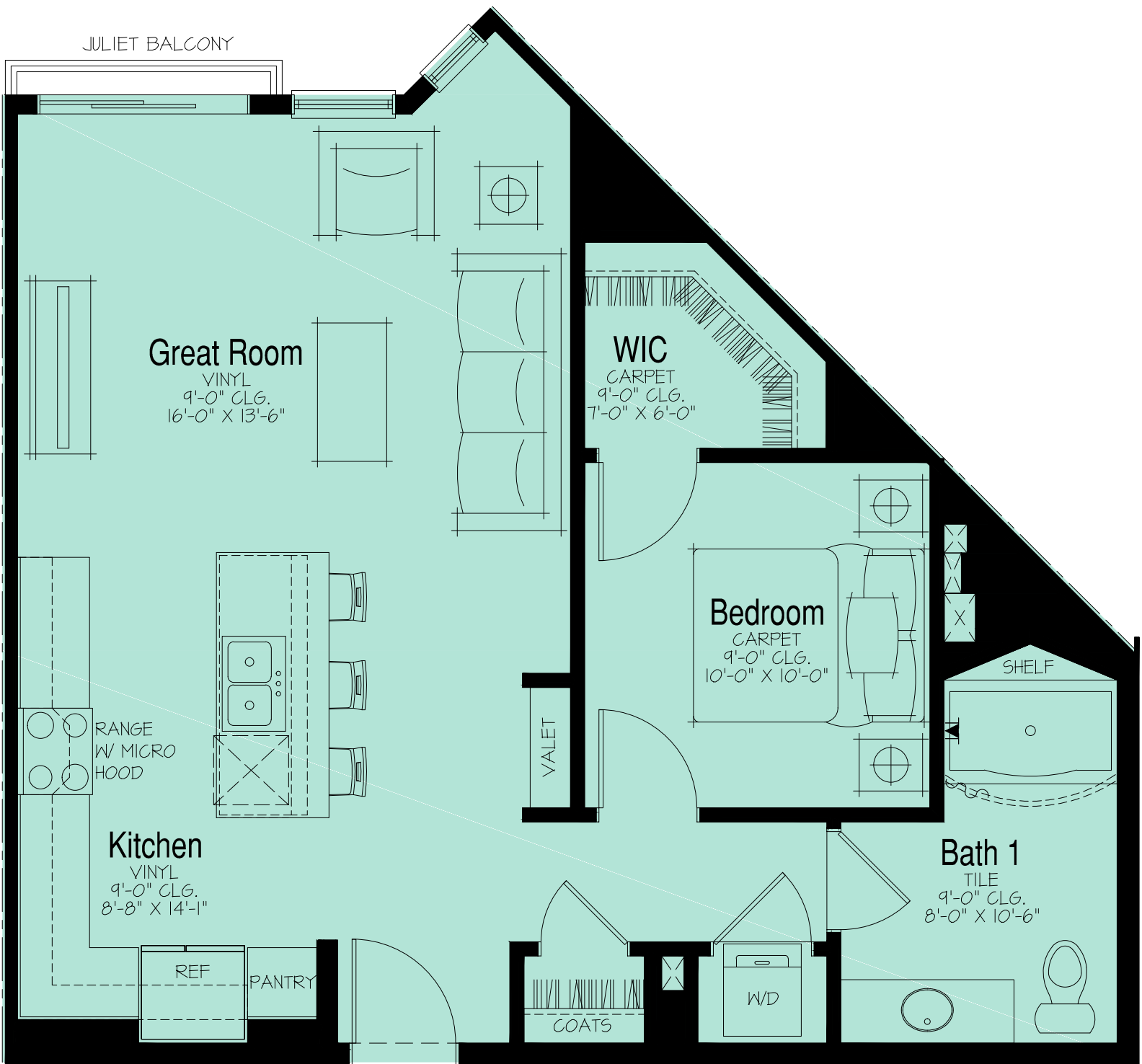
ANSI Type B: 1 Bedroom / 1 Bath NSF: 702 / GSF: 794 Unit - A2 Floor Plan
