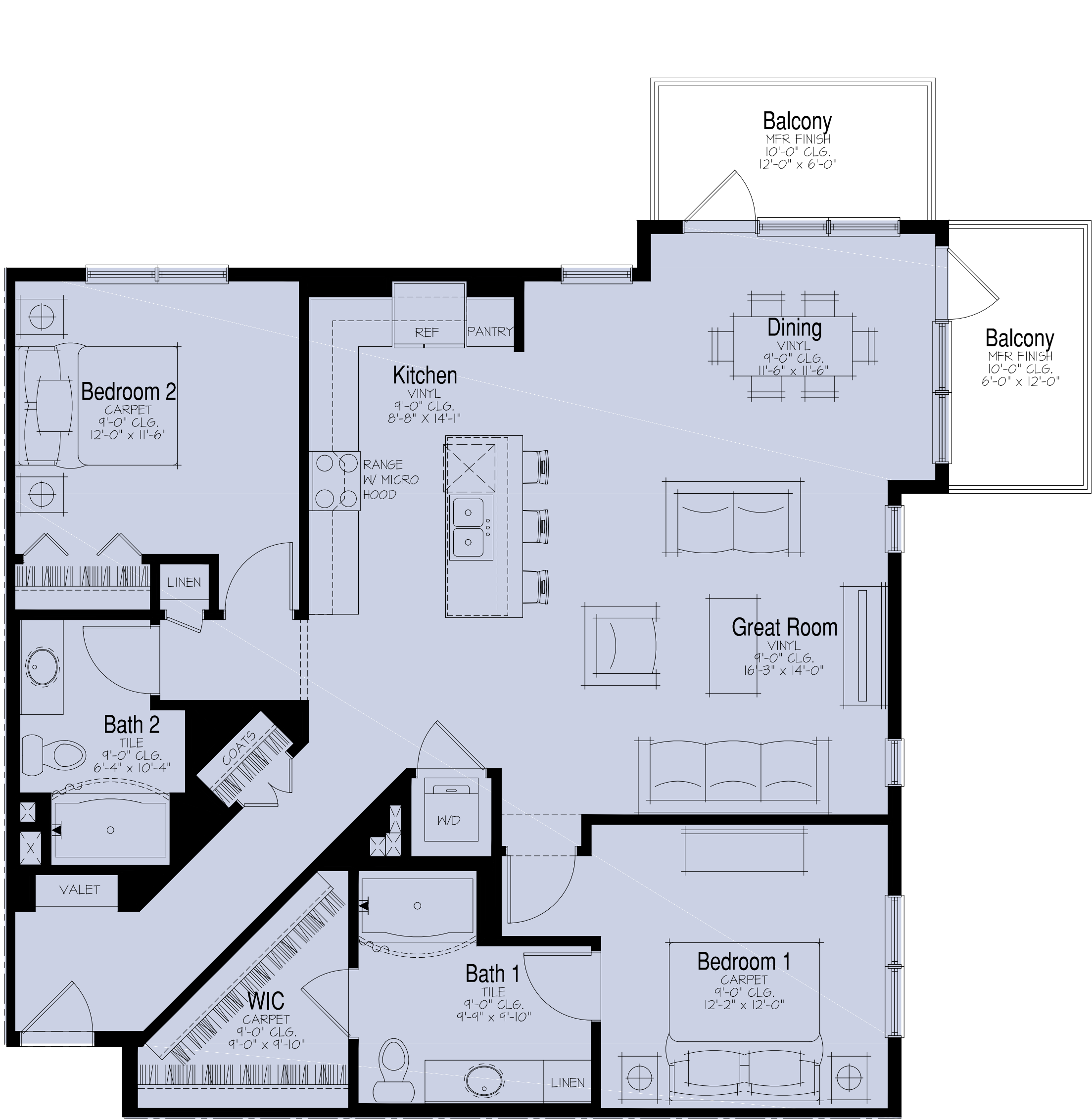
ANSI Type B: 2 Bedroom / 2 Bath NSF: 1288 / GSF: 1382 Unit - B3 Floor Plan SCALE: 1/4"=1'-0" xtr--Unit B3
