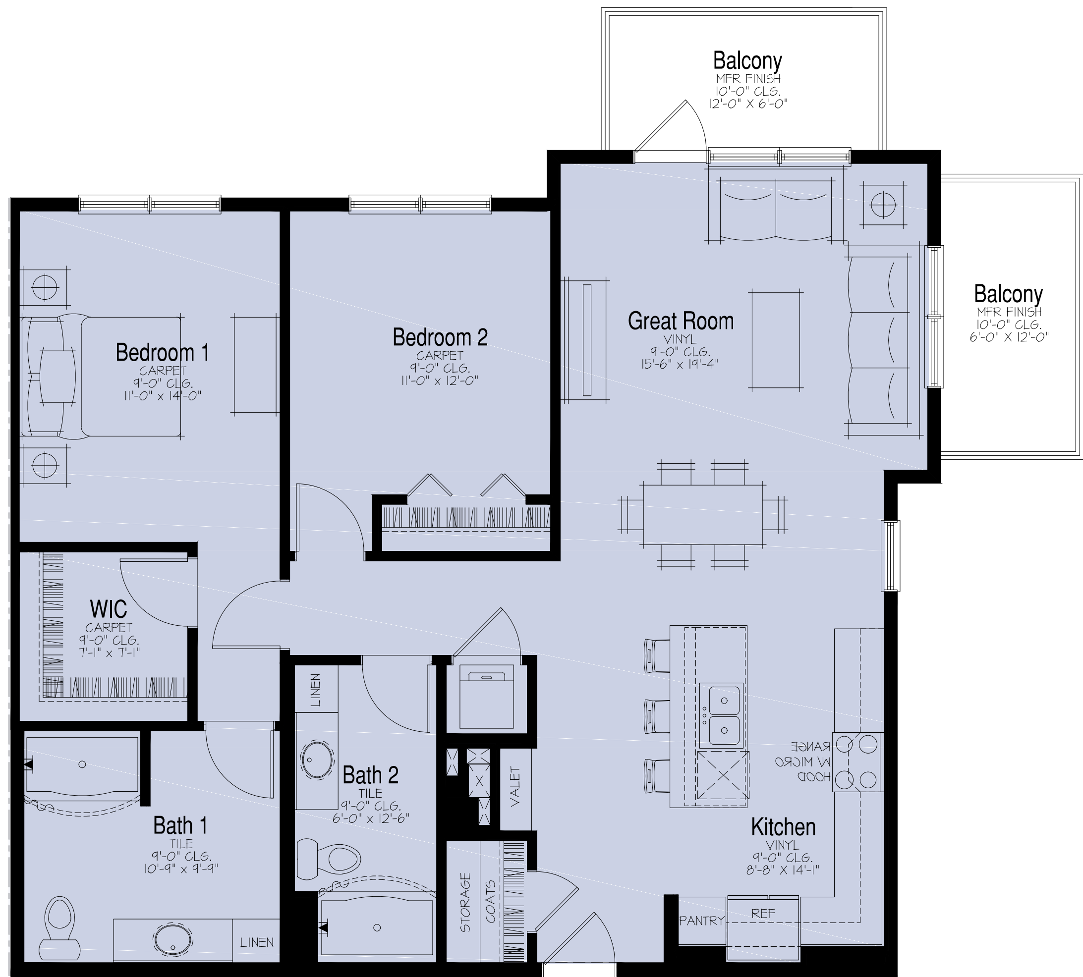
ANSI Type B: 2 Bedroom / 2 Bath NSF: 1198 / GSF: 1276 Unit - B2_Alt Floor Plan
