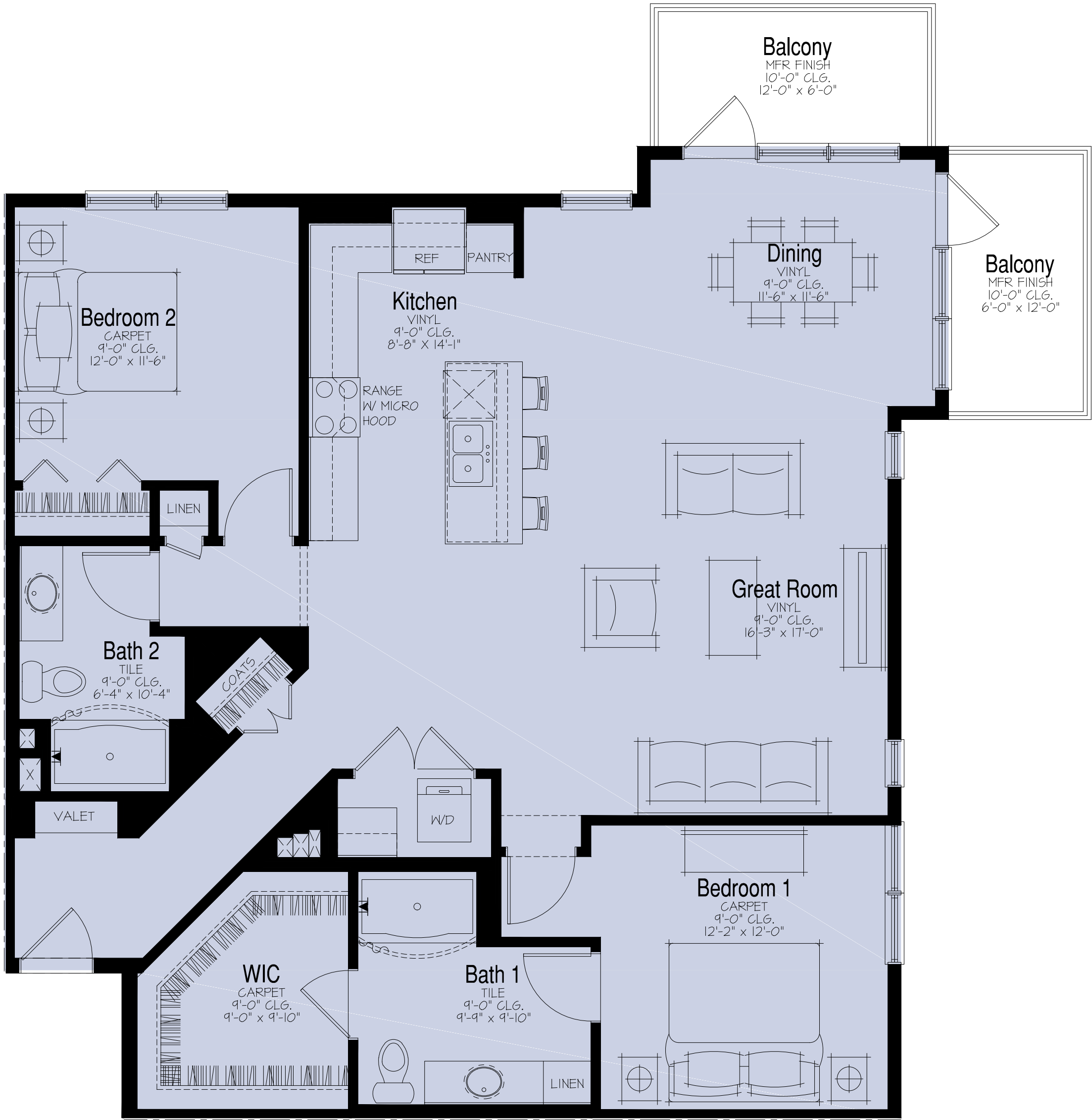
ANSI Type B: 2 Bedroom / 2 Bath NSF: 1398 / GSF: 1484 Unit - B4 Floor Plan SCALE: 1/4"=1'-0" xtr--Unit B4
