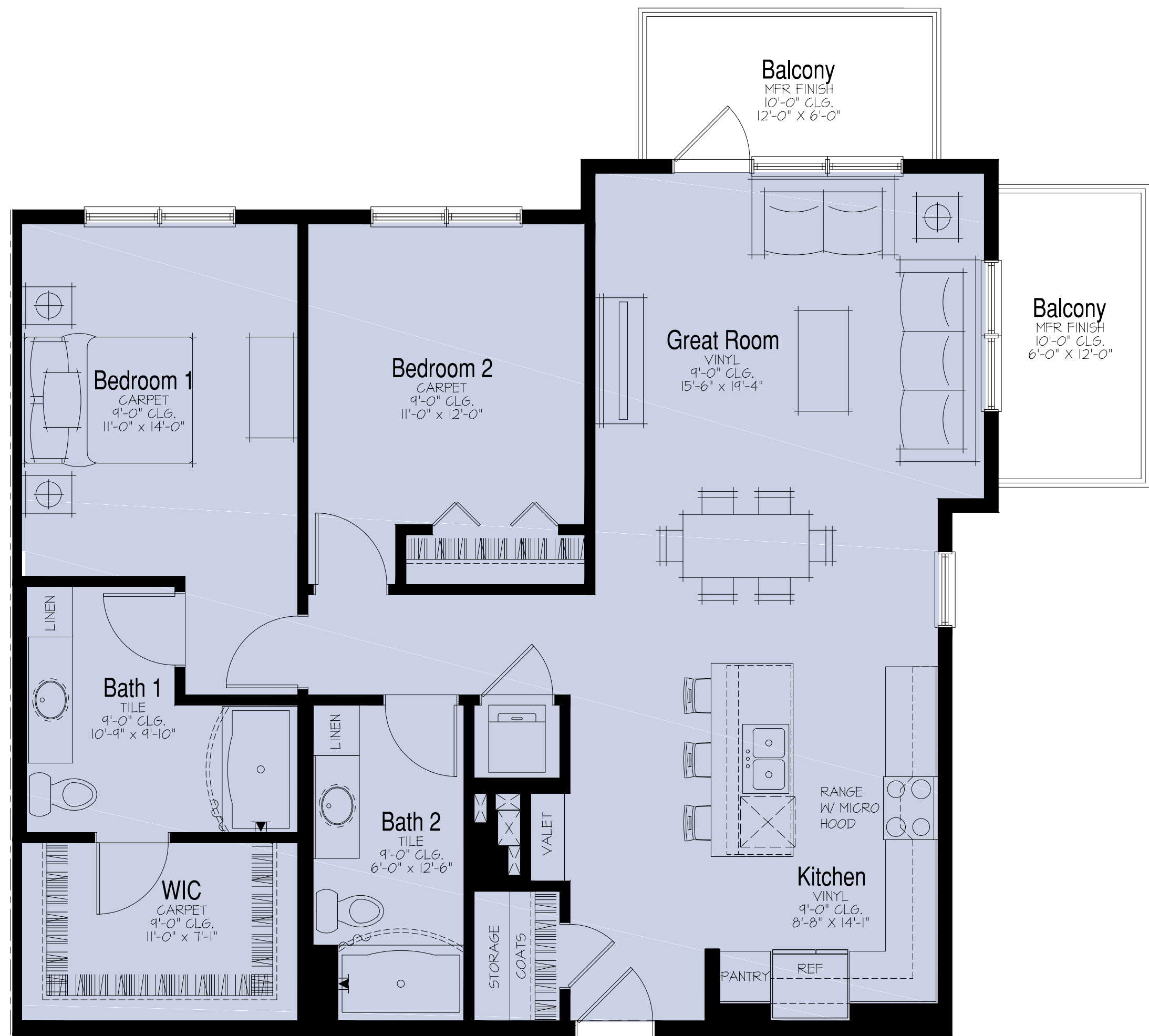
ANSI Type B: 2 Bedroom / 2 Bath NSF: 1198 / GSF: 1276 Unit - B2 Floor Plan
