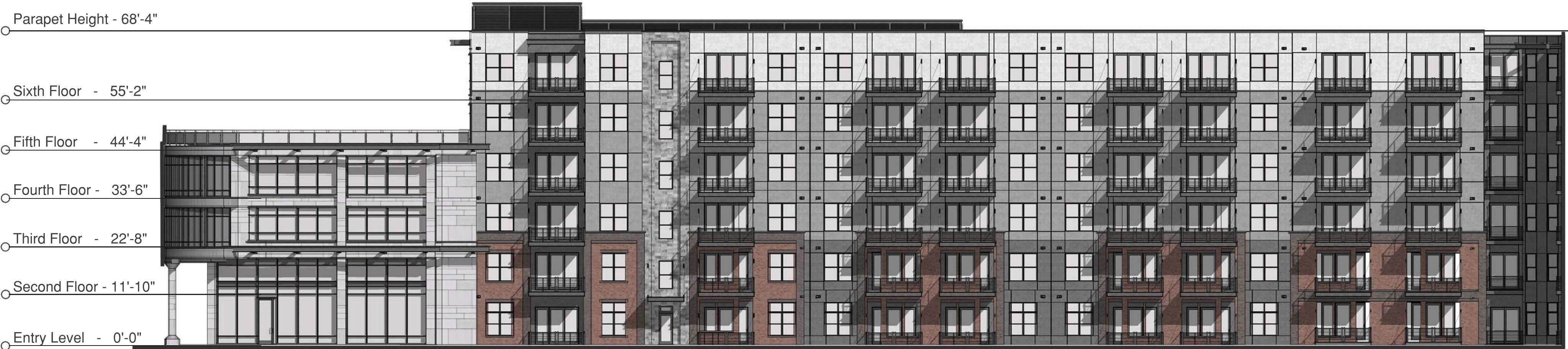
South Courtyard Elevation
