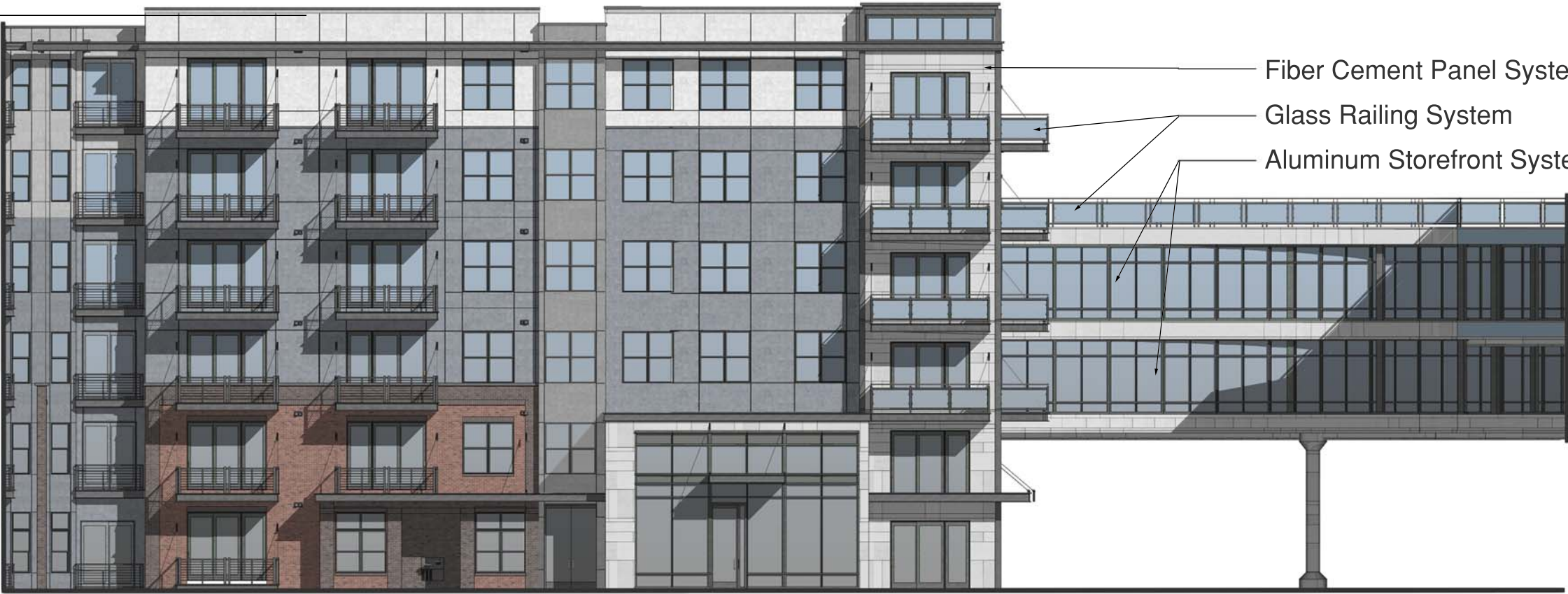
East Courtyard Elevation 1/16" = 1'-0"
