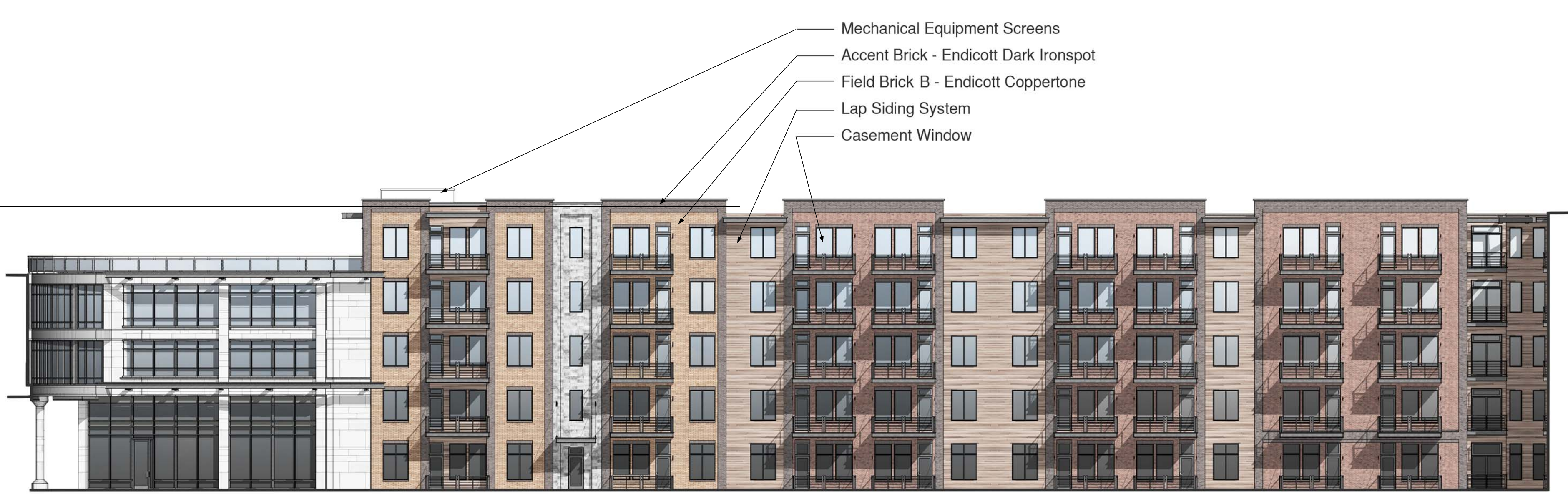
North Courtyard Elevation 1/16" = 1'-0"
