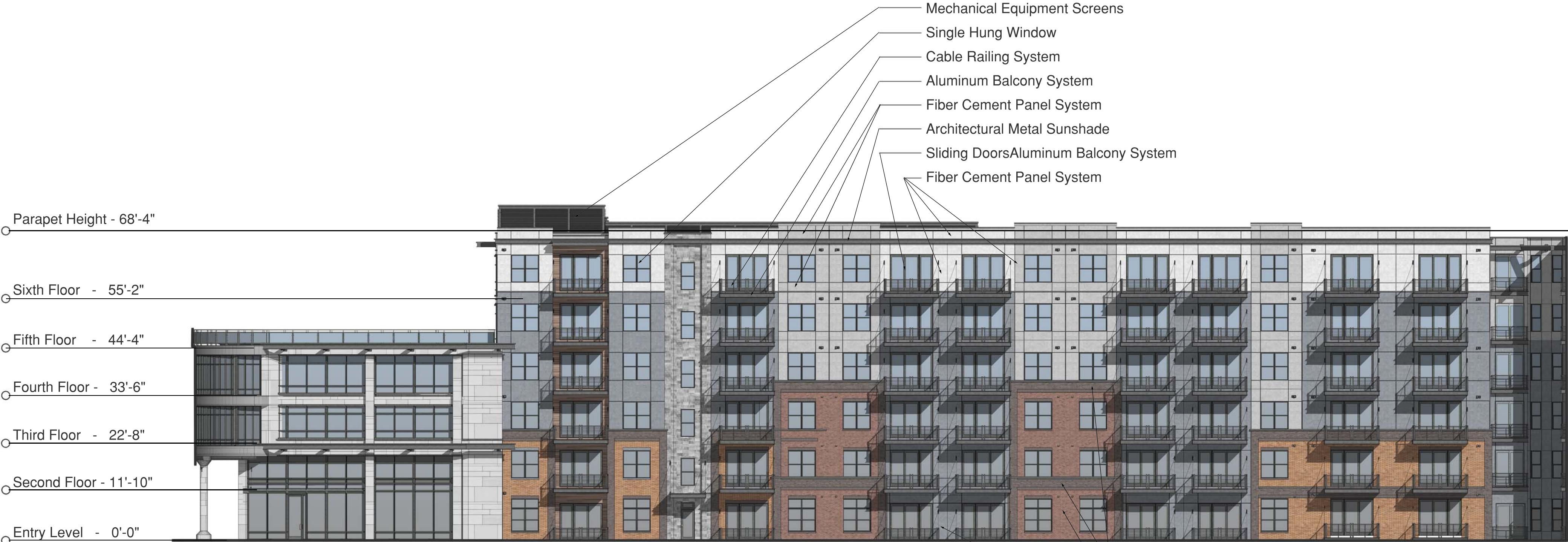
South Courtyard Elevation 1/16" = 1'-0"
