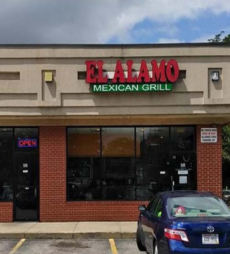
Typical U.L. Channel Letters with LEDs Mounted on Raceway Not to scale
