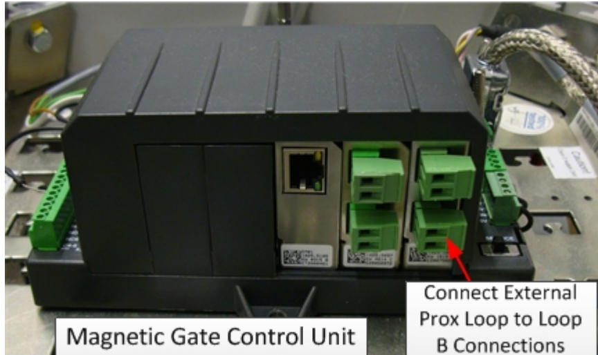
Figure 26. Magnetic Gate Control Unit
